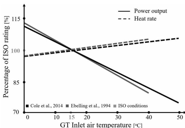
Figure 1. Effect of inlet temperature on GT performance.
