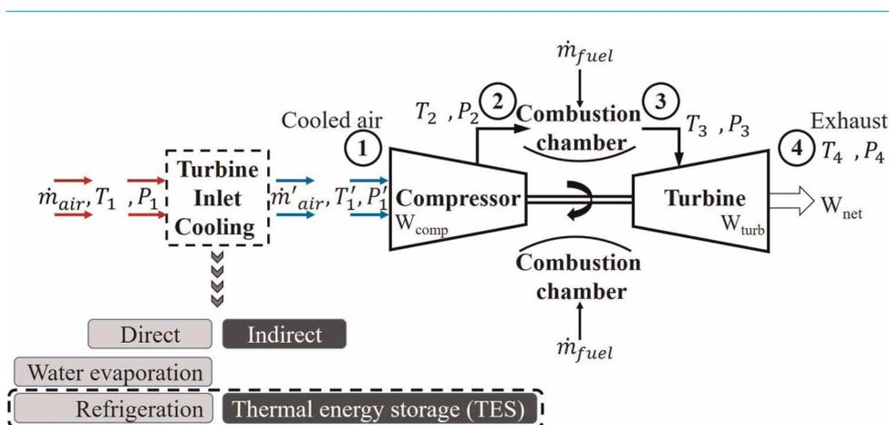
Figure 2. Overview of GT inlet cooling systems.
