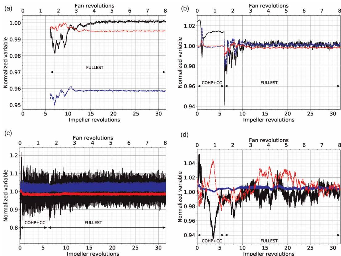
Figure 5. Convergence plots of normalised integral values for (solid black)  $\dot{m}$ , (dash-dotted red)  $T_t$  and (dashed blue)  $P_t$  at four different cross-sectional positions noted in yellow in Figure 1e. Values are normalised by the ones from the thermodynamic cycle. (a) Secondary flow outlet. (b) Impeller inlet. (c) Axial diffuser trailing edge. (d) Combustion chamber exit.
