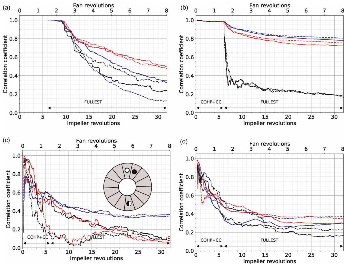
Figure 6. Azimuthal decorrelation plots of local signals for (black)  $u_x$ , (red)  $T$  and (blue)  $P$  at different positions noted in red in Figure 1e. Solid lines represent the decorrelation with the adjacent azimuthal sector whereas dashed lines illustrate the decorrelation with the opposite azimuthal sector. (a) Secondary flow outlet. (b) Impeller inlet. (c) Exit of the axial diffuser. (d) Combustion chamber exit.
