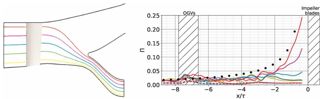
Figure 8. Normalised pressure jump  $\Pi$  at different values of  $h/H$ : (yellow) 10%, (green) 30%, (cyan) 50%, (violet) 70%, (red) 90%. (solid) FULLEST, (dashed) FAN + OGV. (•) analytical expression (Equation 2).
