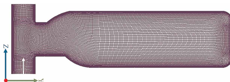
Figure 6. Meridional plane of the numerical grid.
