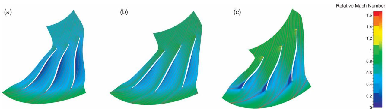
Figure 7. Relative Mach number contours and streamlines of the impeller with a flow coefficient of 0.18. (a) 10% span. (b) 50% span. (c) 90% span.
