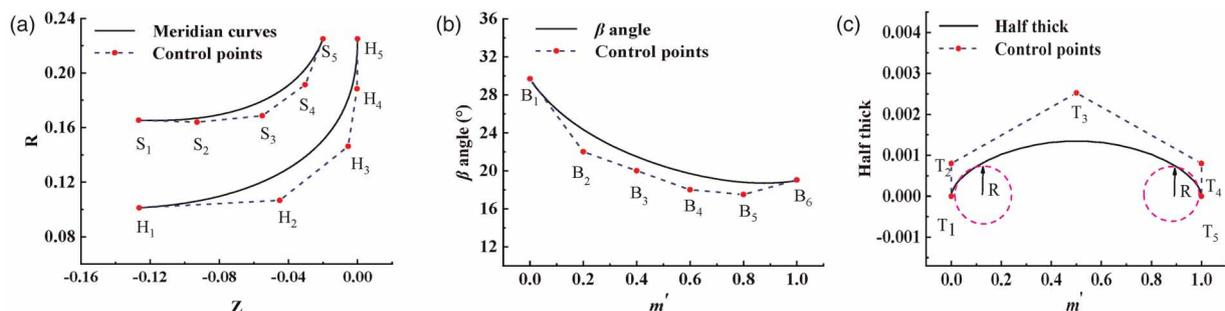
Figure 2. Parameterization model of meridional channel (a),  $\beta$  at the hub (b), and thickness at the hub (c).
