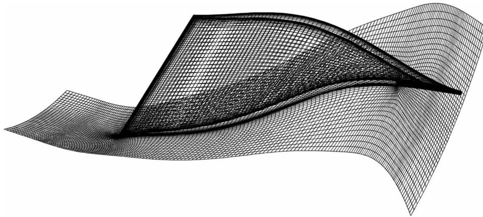
Figure 3. Surface grid of the impeller.
