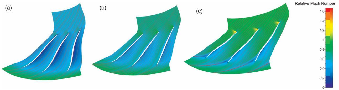
Figure 9. Relative Mach number contours and streamlines of the impeller with a flow coefficient of 0.22 (a) 10% span (b) 50% span (c) 90% span.
