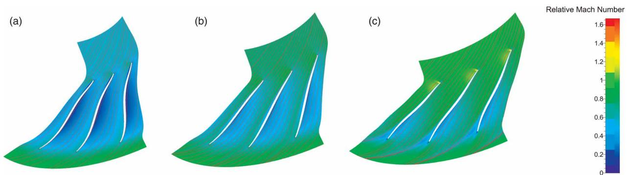
Figure 8. Relative Mach number contours and streamlines of the impeller with a flow coefficient of 0.2. (a) 10% span. (b) 50% span. (c) 90% span.
