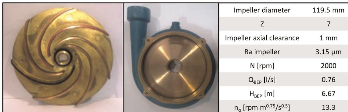
Figure 2. Pump tested.
