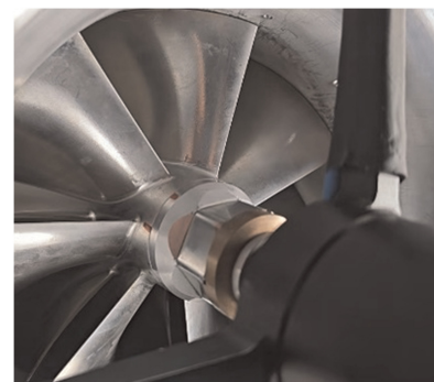
Figure 10. Loosening of the centrifugal impeller locking nut.
