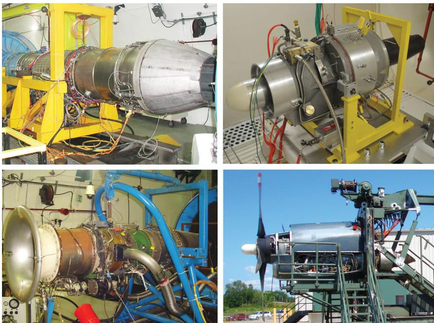
Figure 1. The four engines platforms used for testing. Clockwise from top left: F-404-400; TRS-18-046-1, T-56-A15; and CF-700.
